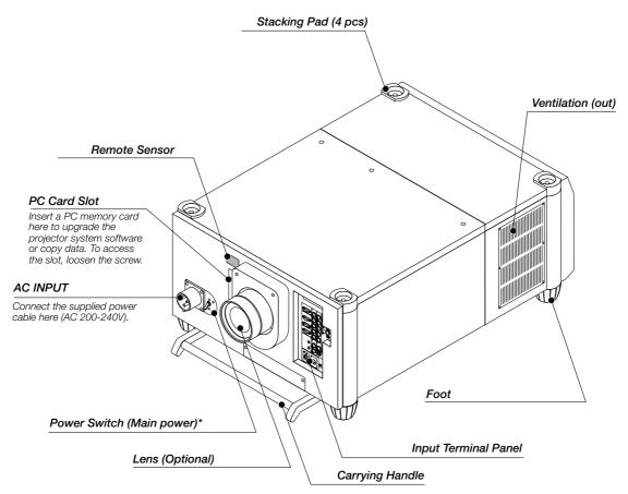
\* To turn on the main power to the projector, press the switch to the ON position (I) and the POWER indicator on the rear panel will turn orange in color.
